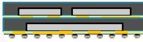
Two Laminated Layers and Side Metal Interconnect
